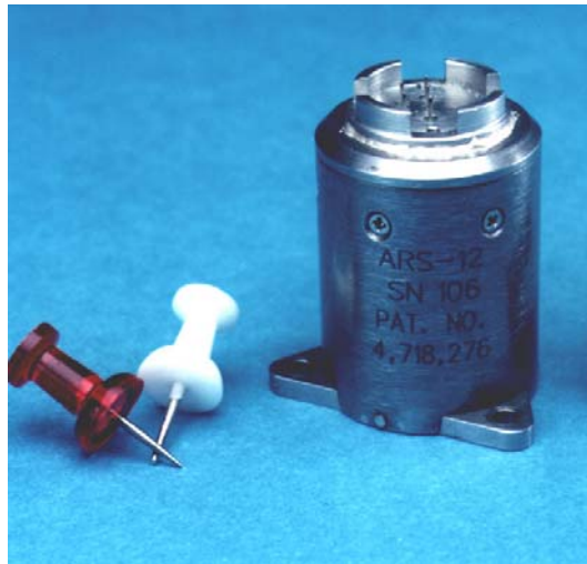
Figure 2 Photograph of High Performance MHD Angular Rate Sensor
